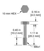
M6x1 Captive Bolt, for CTC M/AC194 and M/AC294 Sensors, 18-8 Stainless Steel, 1.11 in. (28 mm) Length
