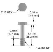
1/4-28 Captive Bolt, for CTC AC194 and AC294 Sensors, 18-8 Stainless Steel, 1.11 in. (28 mm) Length
