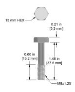
M8x1.25 Captive Bolt for Standard Size Side Exit Accelerometers, 18-8 Stainless Steel, 1.48 in. (38 mm) Length
