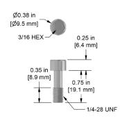
1/4-28 Captive Bolt Socket Head Cap for CTC Miniature Industrial Side Exit Sensors, 18-8 Stainless Steel, 0.75 in. (19 mm) Length
