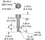
10-32 Adapter Bolt with Socket Head Cap for CTC AC119, AC115, AC230 and AC360 Sensors, 18-8 Stainless Steel, 0.89 in. (22 mm) Length
